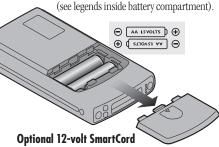
To power Solo S3 using 12-volts, simply remove the power connector plug, and insert the small end of the optional SmartCord, (telephone-type connector) into the modular jack on Solo S3's right side. Plug the lighter plug adapter into your vehicle's lighter socket or accessory socket.
