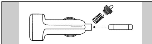
Unscrew the tip of the lighter socket plug carefully when replacing the 2 amp fuse.
