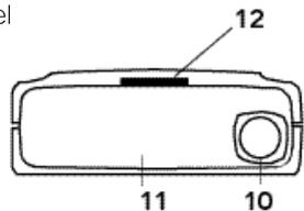
**10. Laser Antenna (Front)** - High gain optical lens provides increased sensitivity and field of view for leading-edge laser detection.
