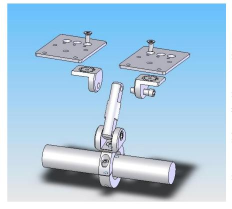
Step 1. Remove the Shaft Pivot Bolt holding the shaft onto the Base Pivot. Use supplied 3/16" hex key. Remove the shaft by lifting straight out. This allows access to a 1/8"head bolt inside the Base Pivot. Note: The Base Pivot can be turned to any direction needed.
