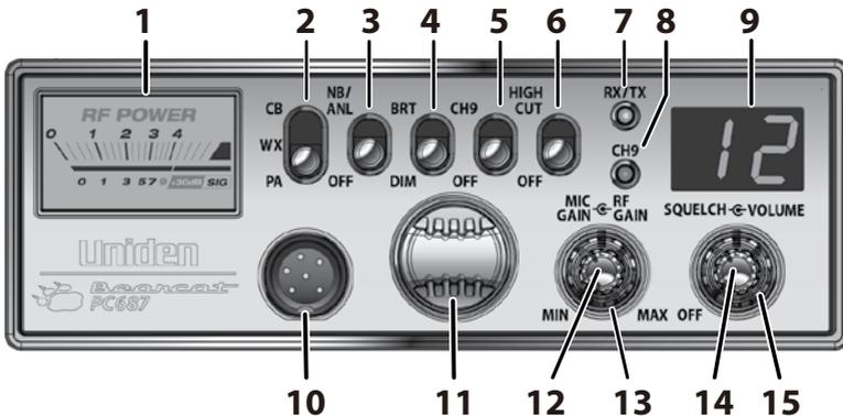
1. **Function** meter. When receiving, the meter shows the received signal strength. When transmitting, the meter shows the output power.
