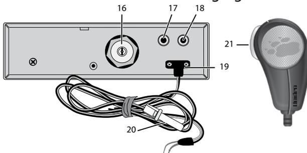
16. Antenna socket: Connects antenna to the unit.
