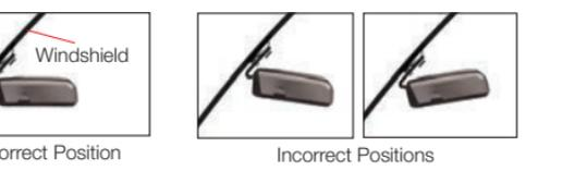
Avoid blocking the detector's view by windshield wiper blades or dark tinting at the top of the windshield.
