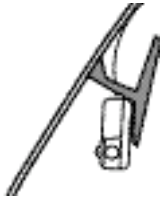
Laser antenna mounted to rearview mirror with Hook & Loop Fasteners.
