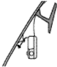
Laser antenna mounted with windshield bracket.
