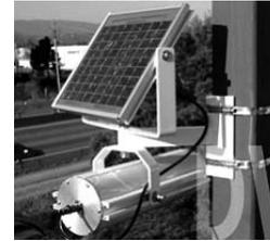
These sensors are fully self-contained and roadside-mounted.
